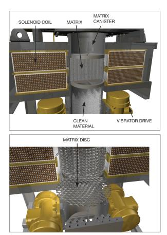
Figures 2 and 3: The DVMF consists of a thick steel box with a canister in the bore. Aluminum or copper coils are positioned around the canister. Direct current power energizes the coil and allows the matrix to collect magnetic particles.
