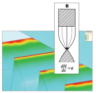
Schematic 1: The DVMF's matrix converges the lines of magnetic flux for improved collection of magnetic contaminants.
