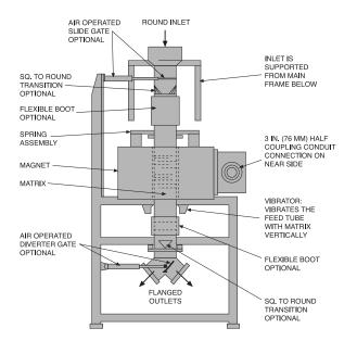
Figure 1: Dry Vibrating Magnetic Filters are designed specifically for dry applications - the treatment of powders. Its purpose is to remove fine ferrous contaminants from dry powder.
