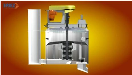
As described in the [animation](#), the StackCell design takes advantage of a patented independent contacting chamber. Feed slurry and air enter this chamber and are subjected to intense shear to generate bubbles and turbulent kinetic energy dissipation rates to promote contacting with the hydrophobic species. Particle collection is achieved in this section and the bubble-particle matrix is subsequently discharged into a quiescent phase separation chamber.
