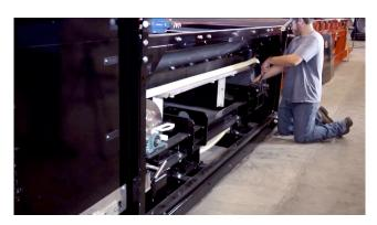
The videos feature RevX-E Eccentric Eddy Current Separators, which are designed with an eccentrically mounted magnetic rotor within a non-conductive shell to separate nonferrous metals. The rare earth rotor produces a powerful and focused field at the end of the belt.
