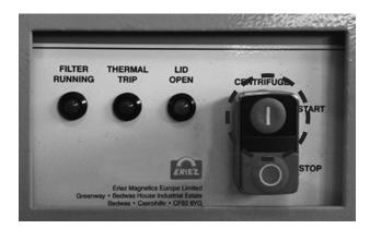
After about 20 seconds, the centrifuge gets up to speed and will able to filter (the centrifuge will not start if the lid is open). Once the centrifuge has been started, start the customer supplied dirty fluid feed pump, or the feed pump supplied on a tank system, to feed fluid to the centrifuge 30-45 seconds after the centrifuge is started.
