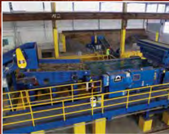
Economical Brute Force Feeder spreads material in this stainless steel recovery operation.
