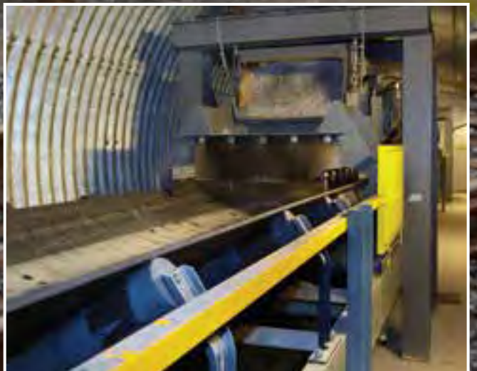
The low profile design of the HVF is ideal for underground installations.
