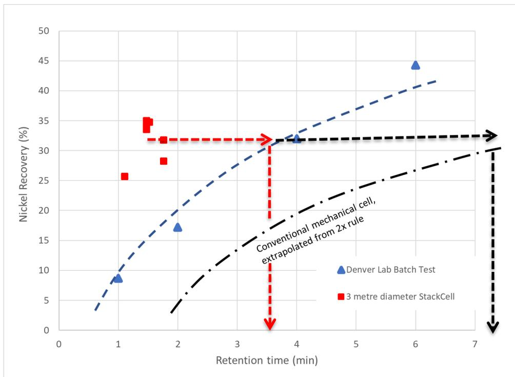
Figure 6. Cleaner kinetic responses for a single 3 metre diameter StackCell and a Denver batch test, based on the same feed
