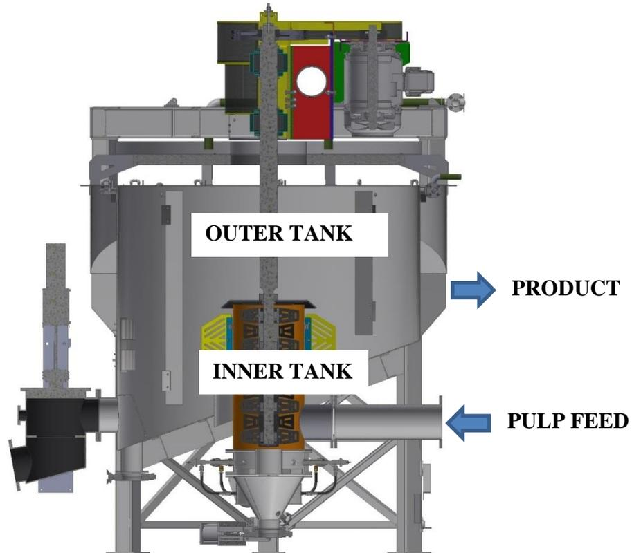
Figure 2. A StackCell cut-away showing the concept of a tank within a tank. The concentric inner tank where particle collection occurs as well as the outer tank, where particle recovery occurs are shown.
