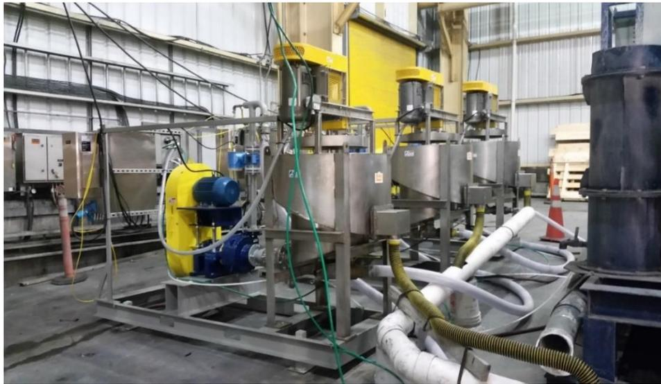
Figure 3. The train of three 0.6 metre diameter StackCells used in this pilot study.
