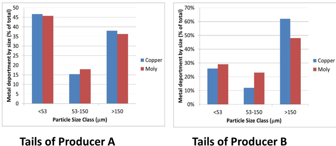
Figure 1. Metal contained in final tailings by size for two major copper concentrators
