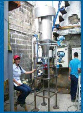
Figure 1: A 16 inch diameter small-scale production HydroFloat™ for gravity tails flotation
